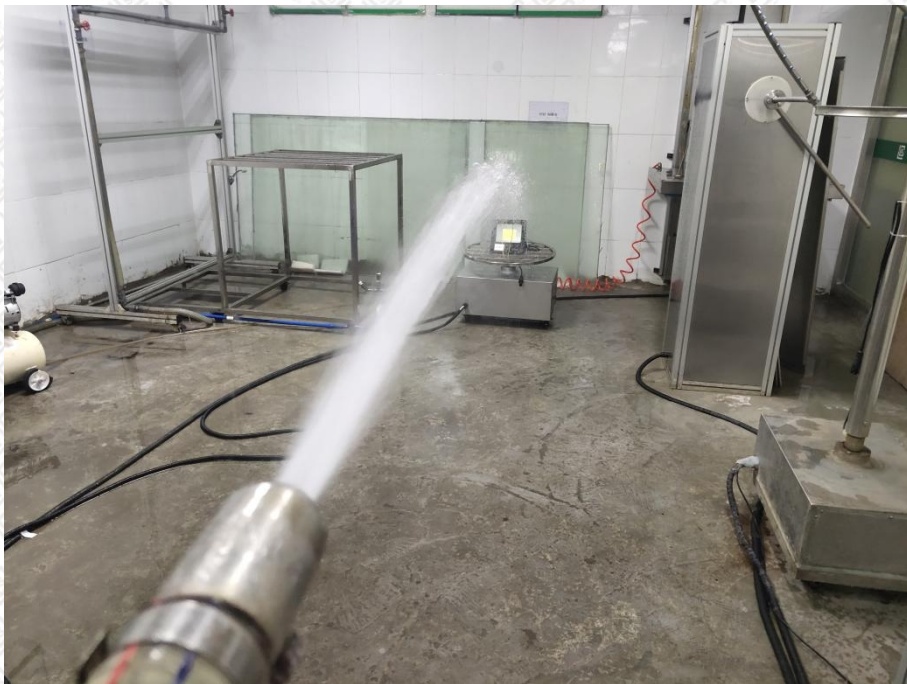
Photo 4: IPX6 test of model 100V2S1COBWW1
