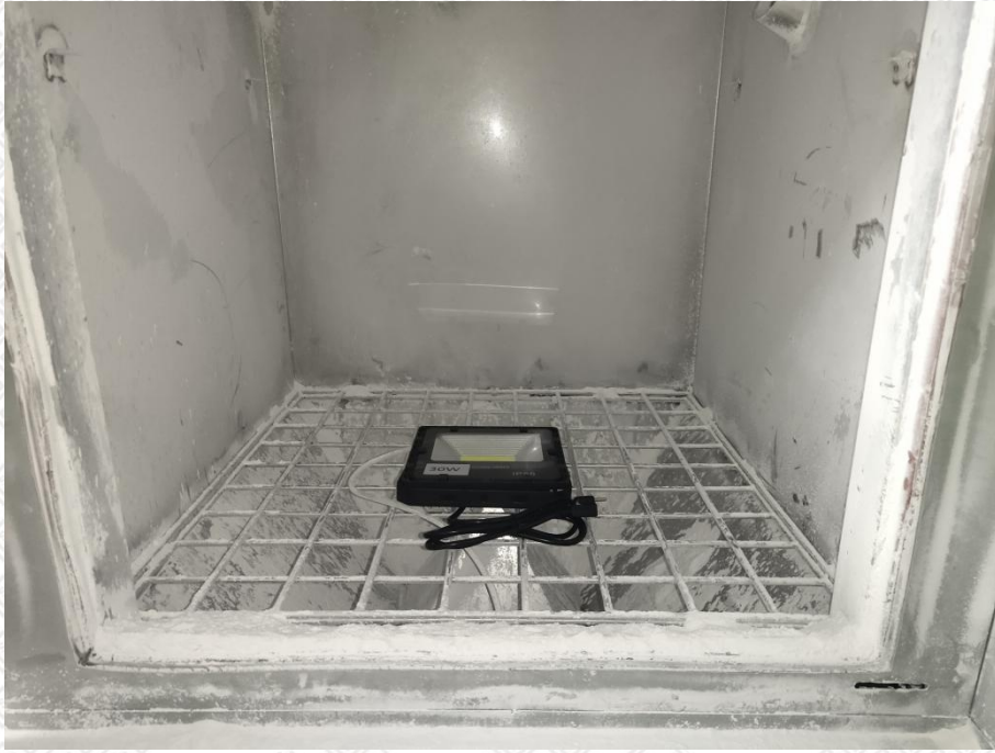
Photo 3: IP6X test of model 100V2S1COBWW1
