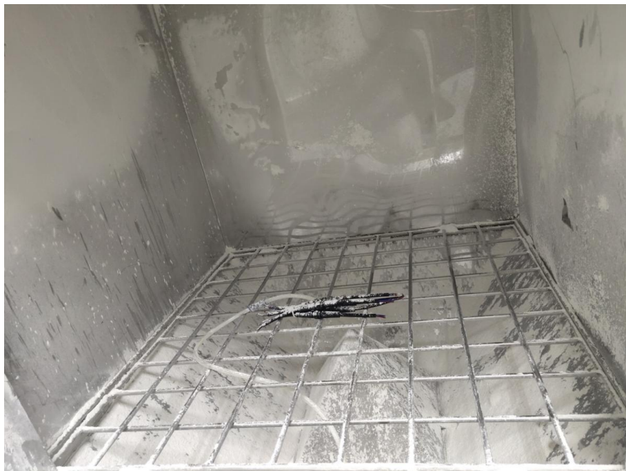
Photo 2: IP6X test of model CONNECTOR II
